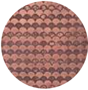
H2 DeErosion su rame DeErosion on copper
